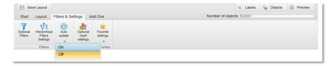
Note: The auto update logic is only applied in "Preview" mode and not in setup mode. In setup mode the Administrator still have to click Update to apply a filter selection even if the Auto update setting is set to On.
